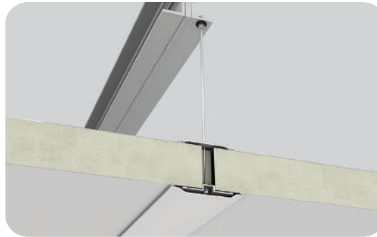
Cold Room Suspender Tiji Detail-2
