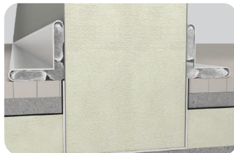
Cold Room Inner Corner Detail
