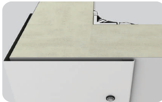
Cold Room Outer Corner Detail-1
