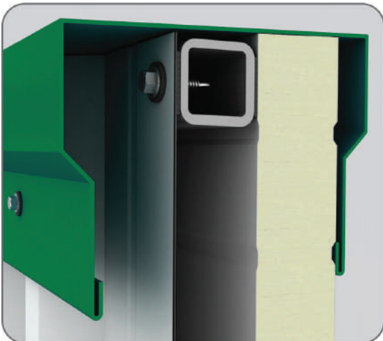
Wall-Roof Connection Detail
